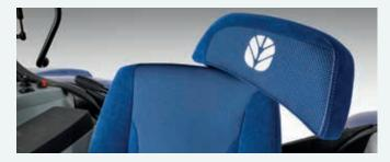
Auto Comfort™ seat All seats benefit from innovative swiveling backrest, designed to provide upper back support and significantly increases comfort The ventilated Auto Comfort™ seat offers a premier seating when the seat is turned to monitor rear mounted implements.
