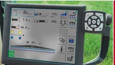
The Leeb GS can be controlled via various external terminals and joystick or the multifunction controler of the tractor.
