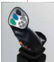
Control by MX loader monolever
