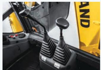
• Conventional pilot controls for the backhoe provide good feedback and response from the hydraulics
